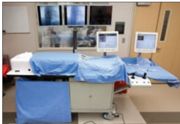
Figure. Samantha endovascular simulator being used to perform coronary angiography. The monitors provide fluoroscopic images and hemodynamic data.
