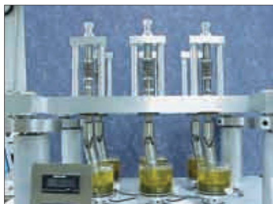
Figure 2. Wear-testing machine designed by the Mayo Clinic biomechanical orthopedics lab to test wear characteristics.
