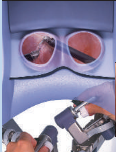
Figure 4. Magnification of 10 times or higher combined with 3-D vision produces a more detailed view of the surgical field, thus increasing surgical precision.
