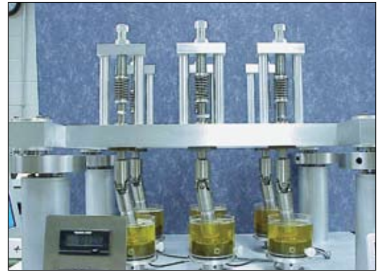
Figure 2. Wear-testing machine designed by the Mayo Clinic biomechanical orthopedics laboratory to investigate wear characteristics.
