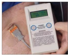
**Figure.** An external electronic stimulator is attached via wires through the skin to 4 electrodes implanted in the diaphragm near the phrenic nerves. The device generates an electric impulse that triggers the diaphragm to contract and allows air to fill the upper and lower parts of the lungs.
